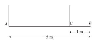
A beam *AB* has mass 12 kg and length 5 m. It is held in equilibrium in a horizontal position by two vertical ropes attached to the beam. One rope is attached to *A*, the other to the point *C* on the beam, where BC = 1 m, as shown in the diagram above. The beam is modelled as a uniform rod, and the ropes as light strings.
