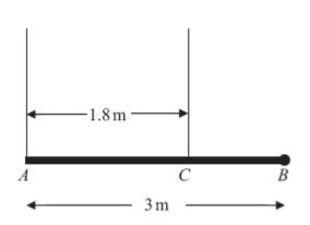
A pole *AB* has length 3 m and weight *W* newtons. The pole is held in a horizontal position in equilibrium by two vertical ropes attached to the pole at the points *A* and *C* where AC = 1.8 m, as shown in the diagram above. A load of weight 20 N is attached to the rod at *B*. The pole is modelled as a uniform rod, the ropes as light inextensible strings and the load as a particle.
