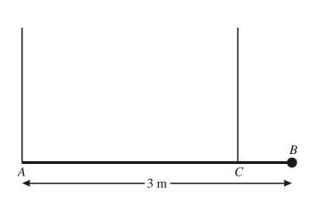
A plank AB has mass 40 kg and length 3 m. A load of mass 20 kg is attached to the plank at B. The loaded plank is held in equilibrium, with AB horizontal, by two vertical ropes attached at A and C, as shown in the diagram. The plank is modelled as a uniform rod and the load as a particle. Given that the tension in the rope at C is three times the tension in the rope at A, calculate
